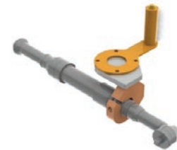
Universal mount allows for setting the torque in any direction.
